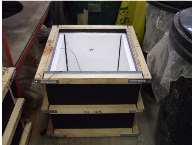
Figure 4 350mm x 350mm x 350mm cube-shaped moulds for heat of hydration specimens (Sarker and McKenzie, 2009)
