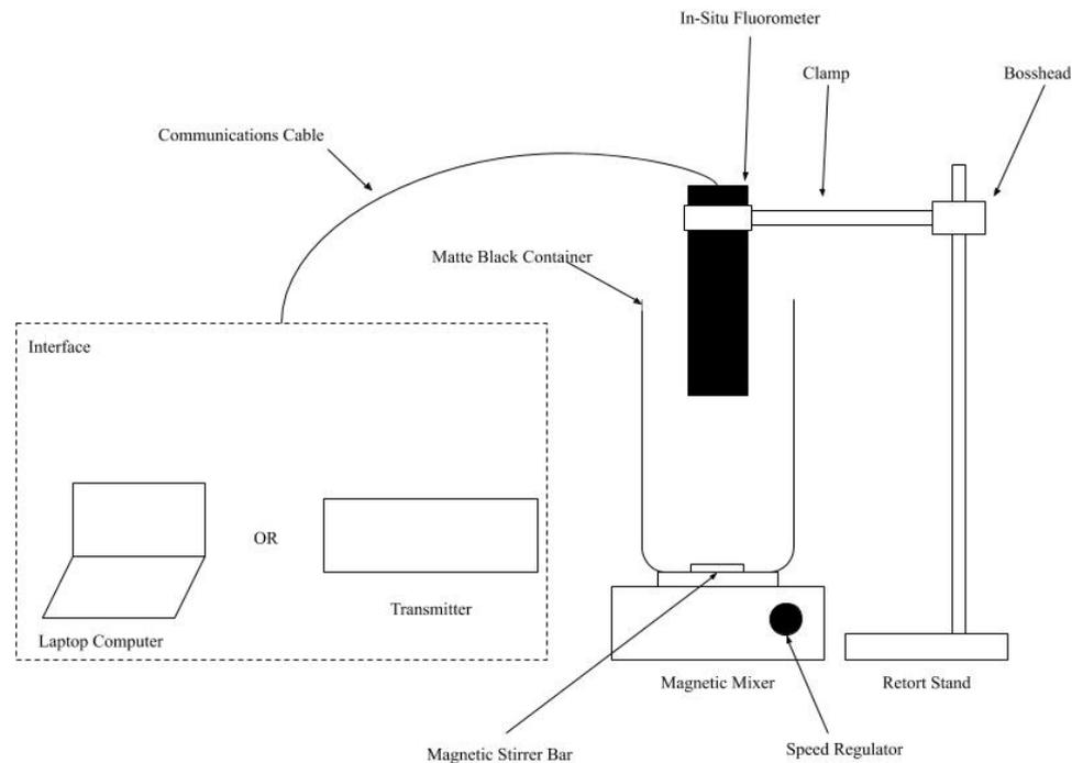
**Figure 1** Experimental apparatus for Produced Formation Water trials.
