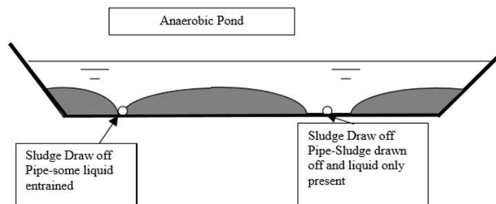
**Figure 5** Typical Sludge Draw-Off Problems from Anaerobic Ponds (Watson, 1999)
