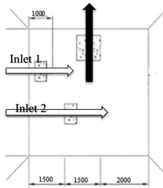
**Figure 1** Inlet pipes (white) and sludge withdrawal (black) pipe configuration at a height of 0.5m from bottom of the smart pond (Water Corporation, 2017).
