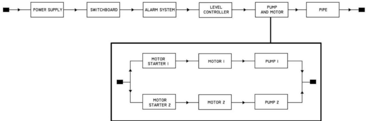
Figure 2 WWPS Reliability Block Diagram
