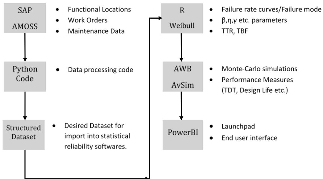
Figure 3 Detailed Data Flow
