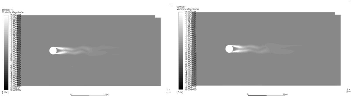
**Figure 4** 2 planes (with 4D separation) plotting vorticity contours, taken from a 3D model of a pipe far from the seabed, with a flow velocity of 2.5 m/s.
