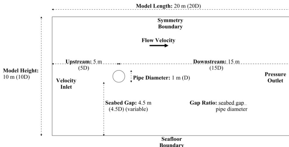
Figure 1 Model geometry and pipe positioning relative to the model extents.
