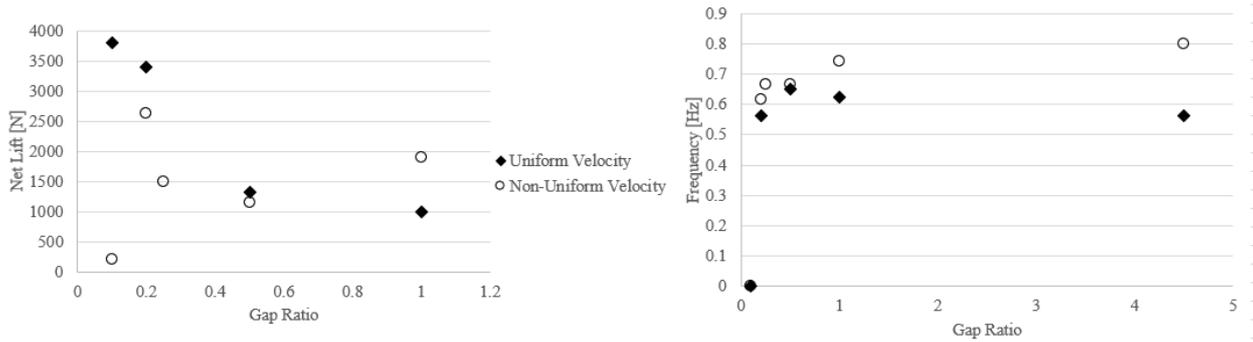
**Figure 3** Vortex shedding frequency and lift force magnitude, for a uniform flow field (diamonds) and a non-uniform flow field (circles).
