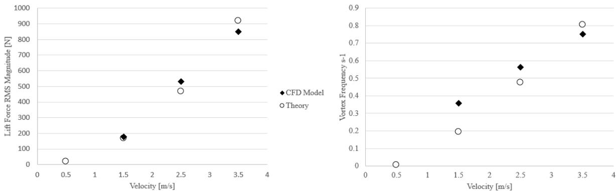
**Figure 2** Plots of (i) the lift force oscillation amplitude and (ii) the vortex shedding frequency, for a 2D model with varying flow velocities.
