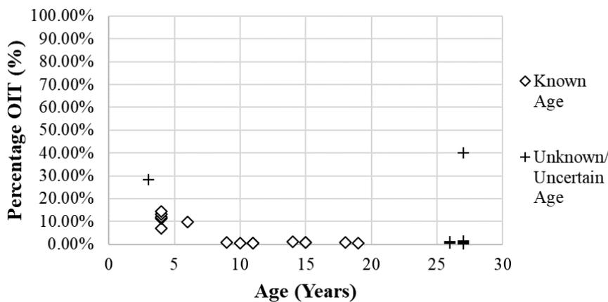
Figure 4 Percentage OIT remaining in samples from failed field samples.
