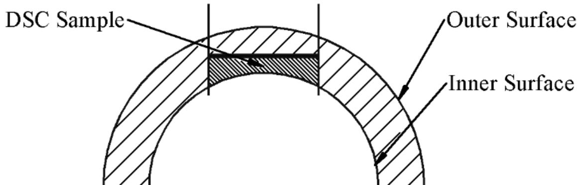
Figure 2 Depiction of DSC sample preparation from pipe cross section.
