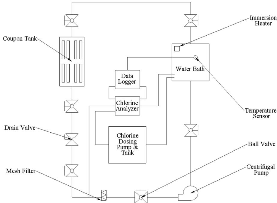
Figure 1 Schematic for pilot test system in AMSI workshop.
