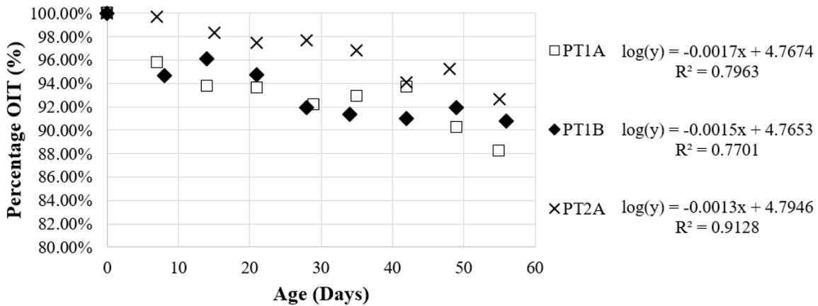
Figure 3 Percentage OIT remaining in samples from Pilot Test 1 and 2.
