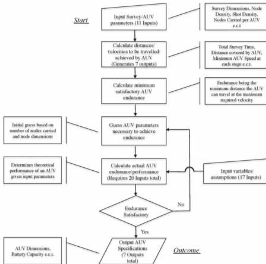
Figure 1 Process implemented in MATLAB to calculate AUV specifications necessary to achieve given design; requiring 31 inputs total. Note - the flowchart is specific to OBN surveys
