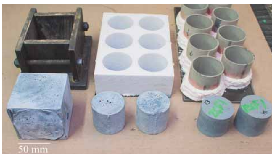
Figure 1 Iterations of mould design left (initial) to right (final): Cube shaped steel mould, Polystyrene cylindrical mould, PVC cylindrical mould. Notice the large improvement in surface finish of the PVC moulds as compared to the others.
