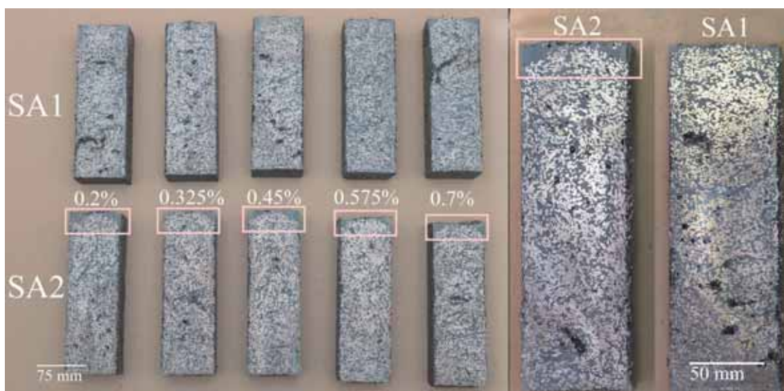
Figure 2 Fibre distribution in brick specimens using suspension agents SA1 and SA2 in amounts varying from 0.2% to 0.7% by mass. The close up on the left shows the difference of fibre sinkage in detail for the concentration of 0.45%. SA2 seems to be ineffective in all cases as seen by the large regions that are missing fibre outlined in the rectangles.
