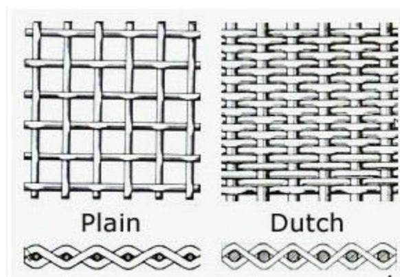
Figure 1 A plain weave compared to a dutch weave wire mesh configuration (Hebei Hangjin Wire Mesh Co., 2016)
