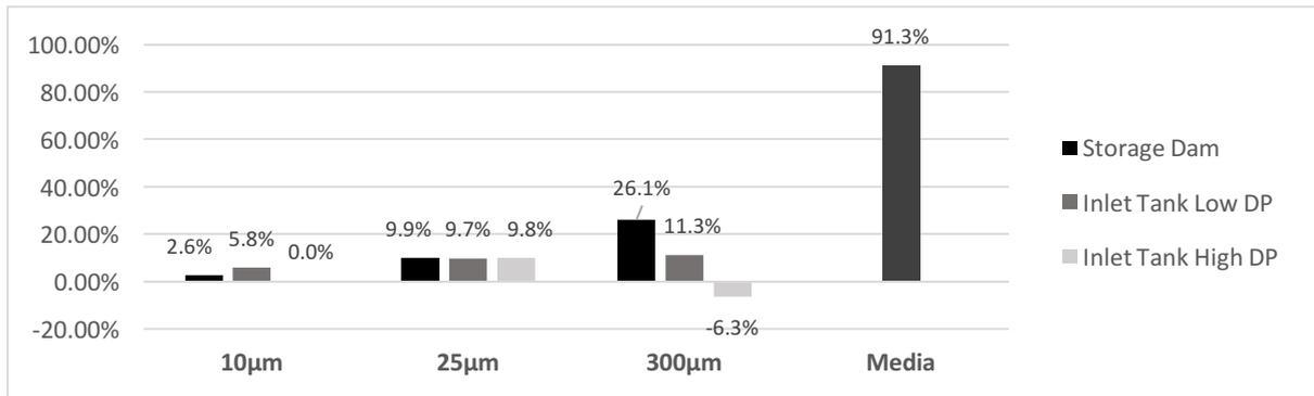
**Figure 3** Algae removal rates at varying mesh apertures, water sources and differential pressure (DP) with media filtration presented for comparison.
