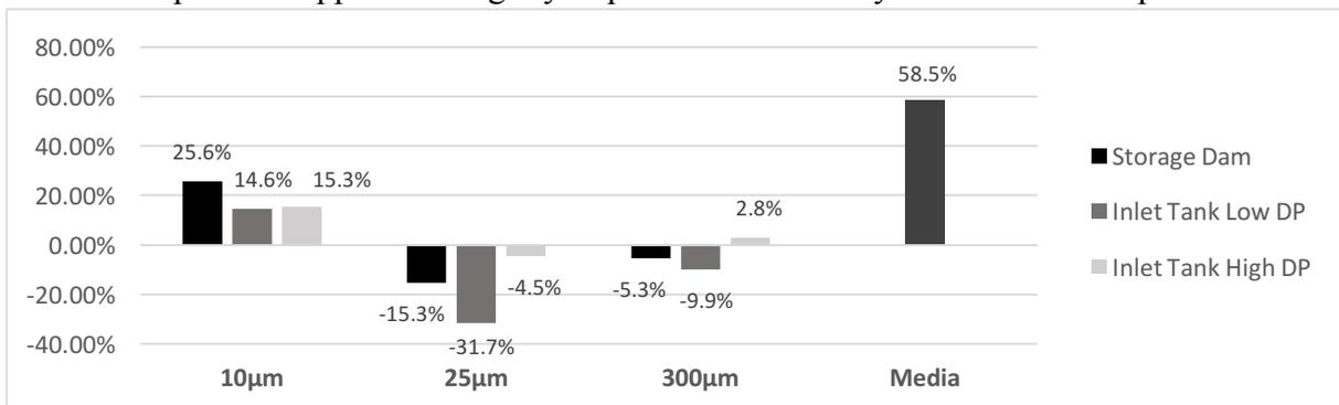
**Figure 2** TSS removal rate at various mesh apertures, water source and differential pressure (DP) with media filtration presented for comparison.
