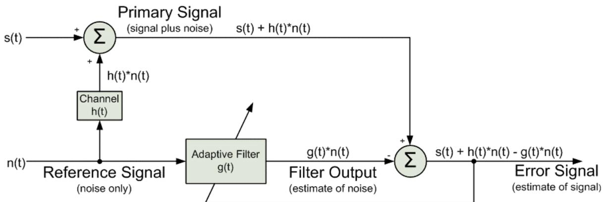
Figure 4 Signal flow in the interference cancellation topology
