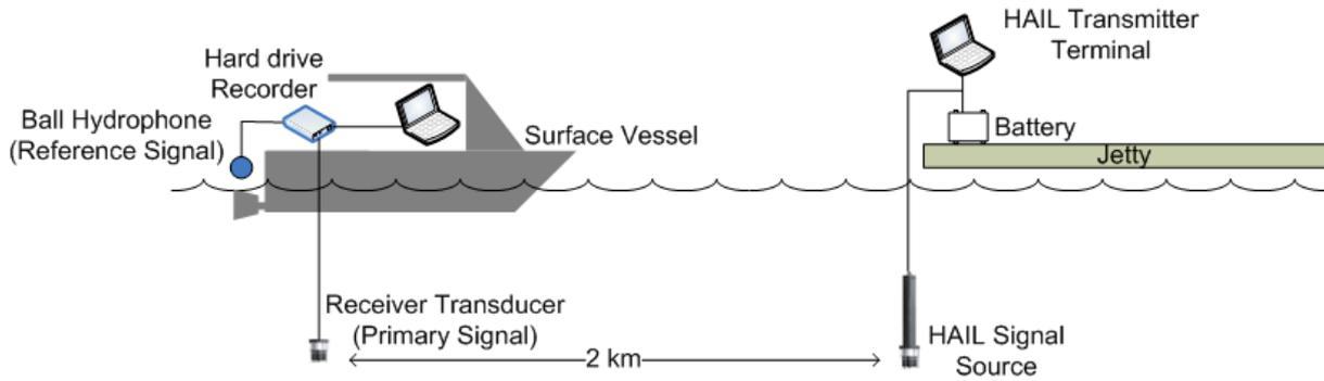
**Figure 6 Trial setup for real data acquisition**
