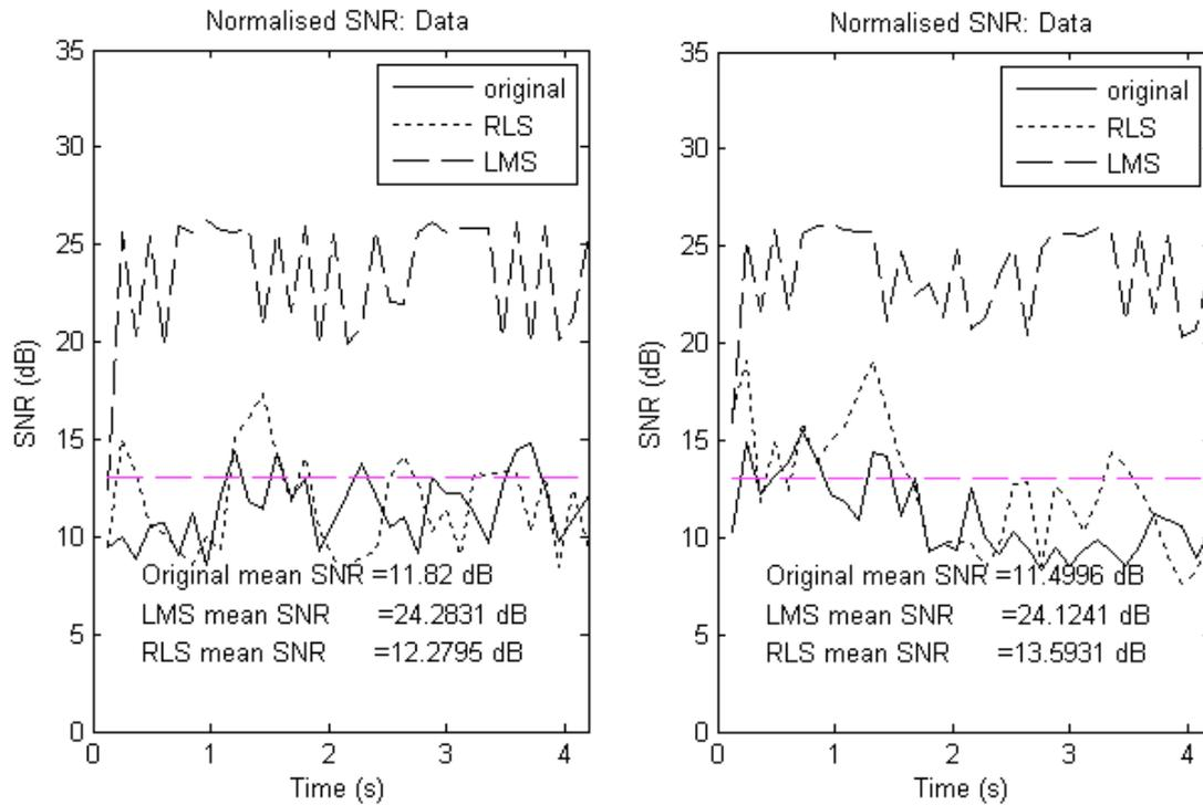
Figure 7 SNR's for (a) Brown noise interference, (b) boat noise interference
