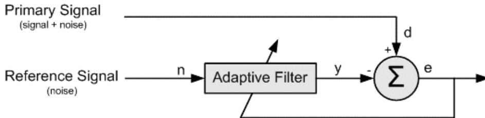
Figure 3 Adaptive filter used in the interference cancellation topology
