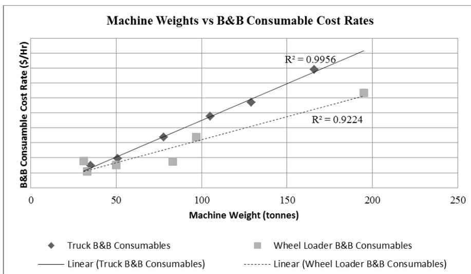
**Figure 1 Model showing the relationship between machine weights and B&B consumable cost rates for trucks and wheel loaders**
