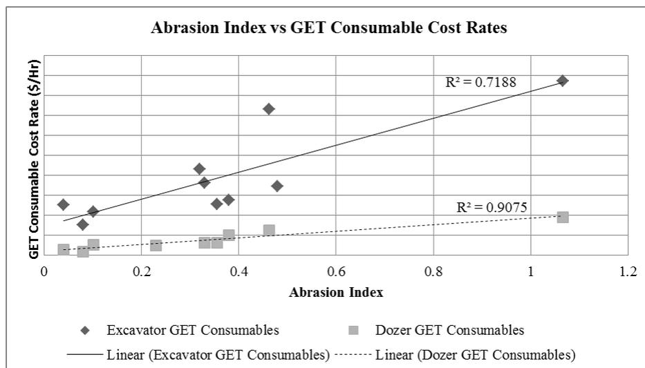
**Figure 2 Model showing the relationship between abrasion index and GET consumable cost rates for excavators and dozers**
