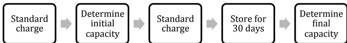
**Figure 2 Self-discharge experiment process flowchart**
