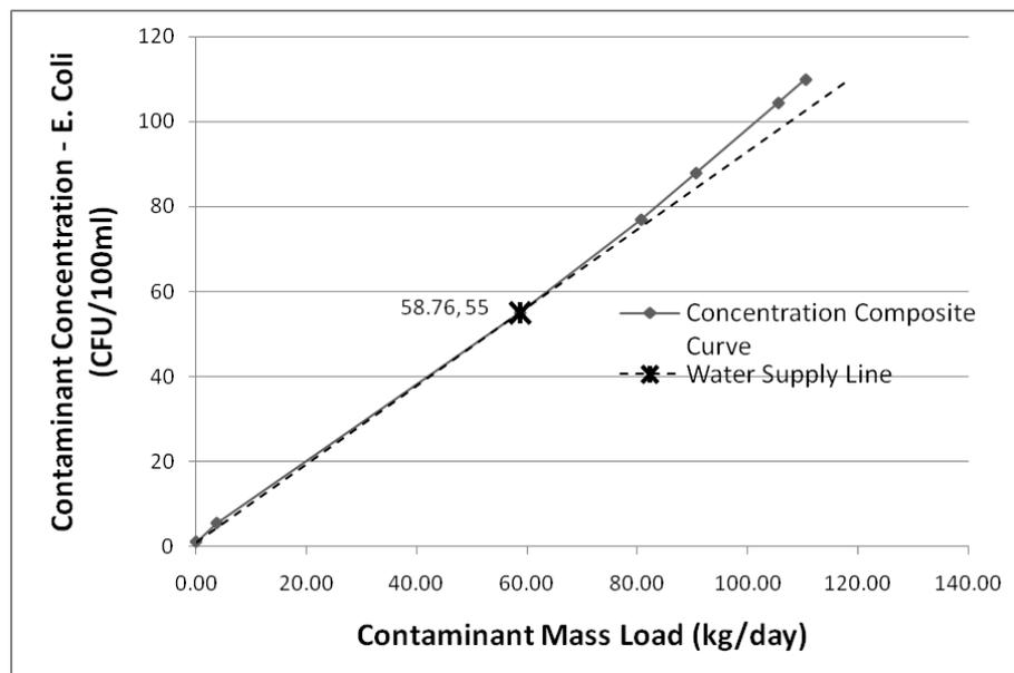
Figure 3 Water pinch analysis on E. Coli of waste streams
