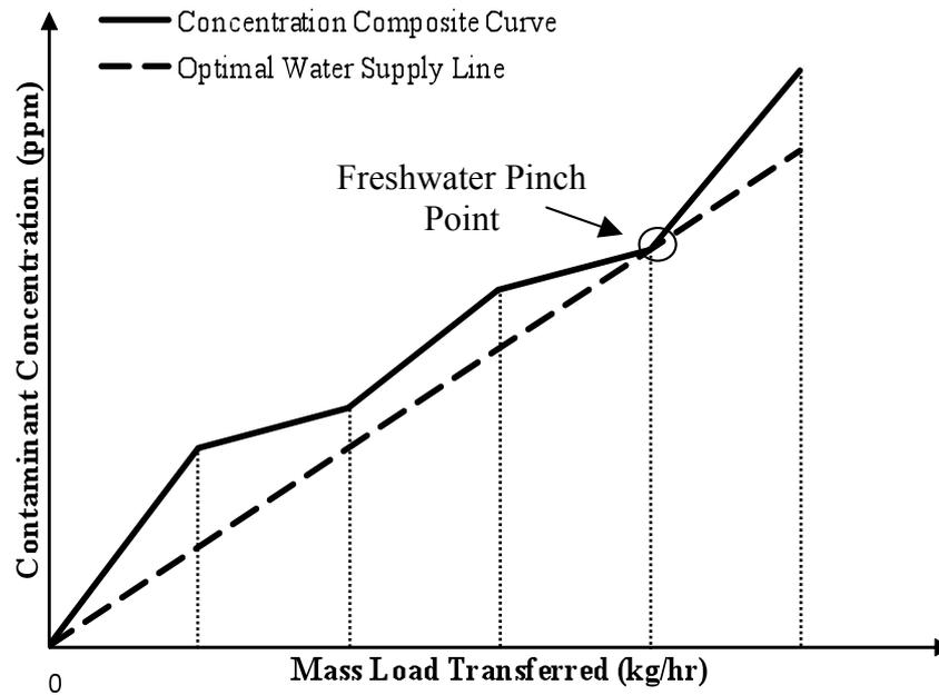
Figure 1 Concentration composite curve and optimal water supply line (Mann and Liu, 1999)
