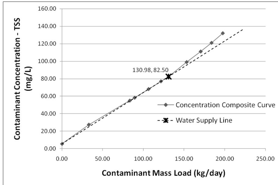
Figure 2 Water pinch analysis on TSS of waste streams
