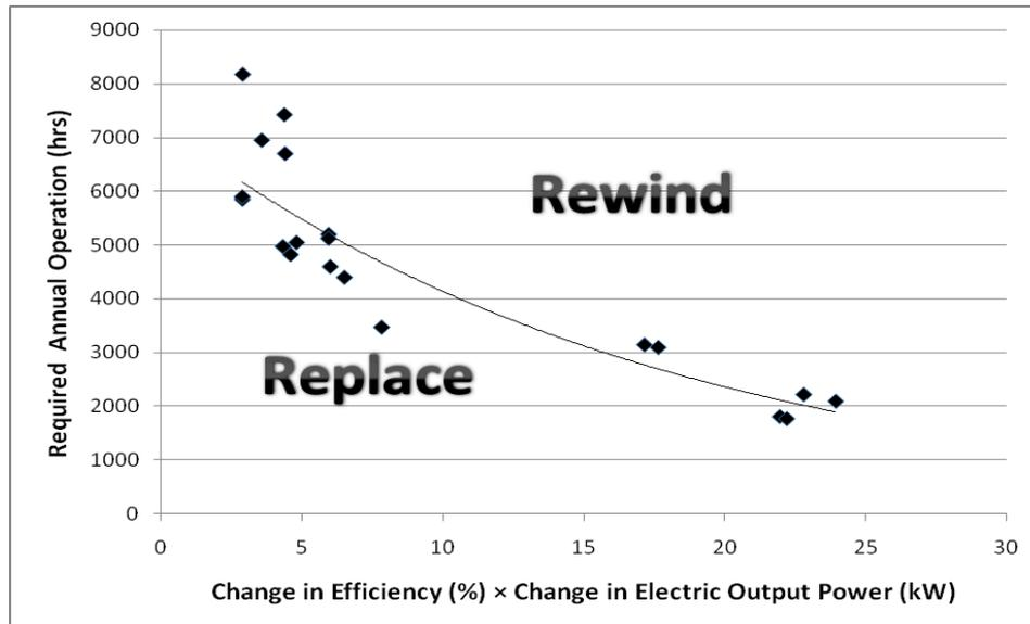
**Figure 1 Relationship between the product of motor efficiency change and electric power change with operating period**
