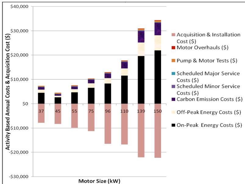
**Figure 2 Activity-based average annual assessed costs incurred by an electric motor (over 25 years) as a function of motor size. Initial Acquisition & Installation Costs depicted below the x-axis.**
