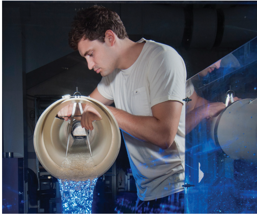
CEED scholar Matthew Avent studying the transport of sand in stratified pipeline flows
