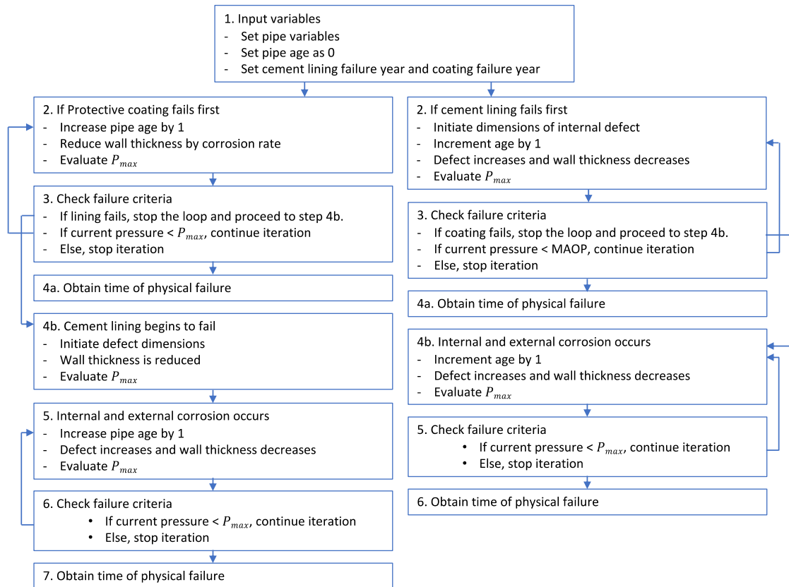
Figure 1 Time to failure model logic diagram
