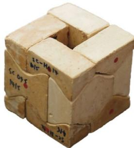
Figure 1: Structure made with osteomorphic blocks (Dyskin, Pasternak & Estrin, 2012).
