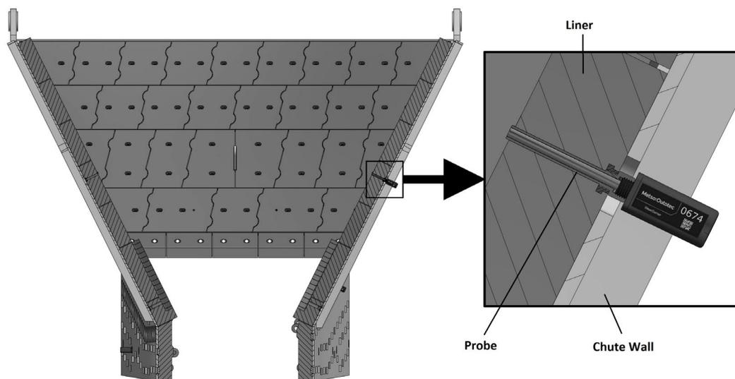
**Figure 1** Schematic representation of a sensor installed on a single liner of a chute.
