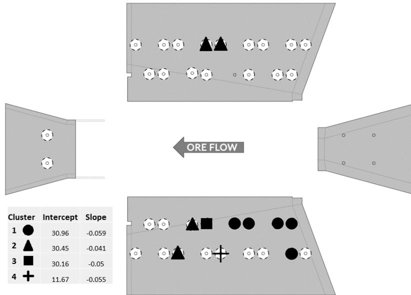
**Figure 3** Clustering results related back to a fold-out schematic diagram of the chute interior (Hopper 1). Each polygon represents an interior panel of the asset. White icons represent non-RUL-0 sensors while the black icons represent RUL-0 sensors with their respective cluster assigned.
