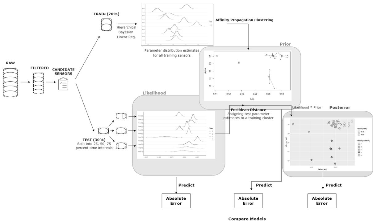
**Figure 2** Process flow diagram representing the entire workflow from raw data to predictions.
