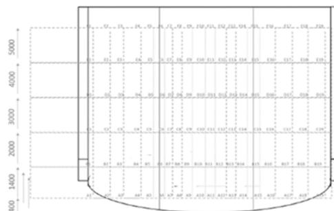
**Figure 1** Thickness Testing Grid (Austin Engineering, 2019)
