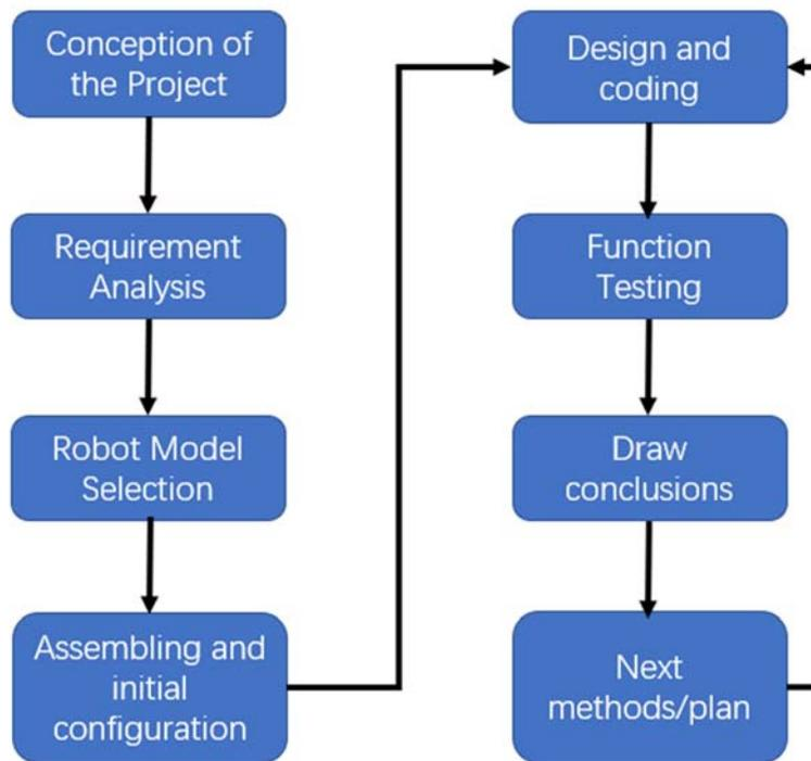
**Figure 2** Overall robot vehicle design process
