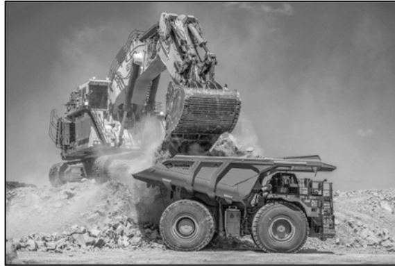
Figure 1 Loading of Austin Engineering's Ultima truck body atop a CAT793F dump truck (Austin Engineering, n.d.)
