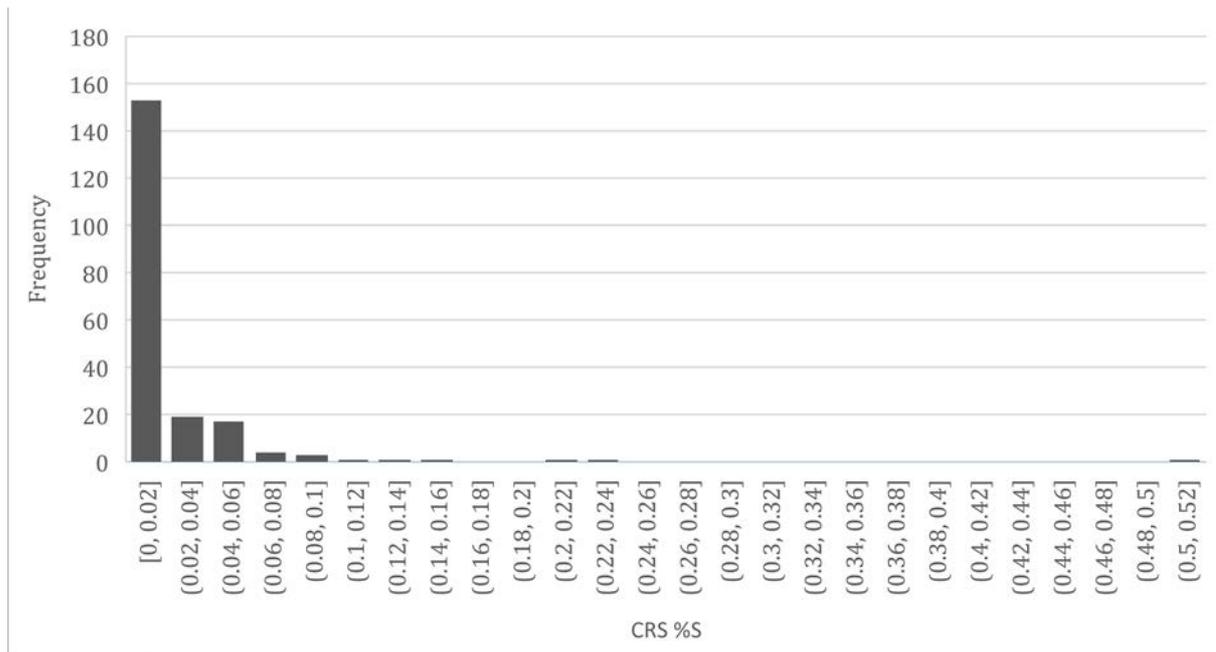
Figure 3 - Percentage Sulfur Distribution based on occurrences. Though the vast majority of data sample have sulfur % below 0.1% some samples had as much as 0.52% sulfur. These outliers are attributed to the presence of other formations and/or coffee rock.
