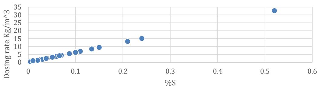
Figure 4 Lime dosing rate (kg/m<sup>3</sup>) trend vs %S. Shows how the dosing rate changes linearly as a function of %S
