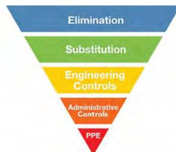
**Figure 1** Hierarchy of Controls (Australia, 2018)
