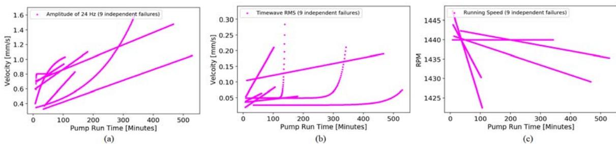
**Figure 5** Trend (exponential fits) of 1X amplitude, RMS of time wave and RPM of pump from station A shown in (a), (b), and (c) respectively
