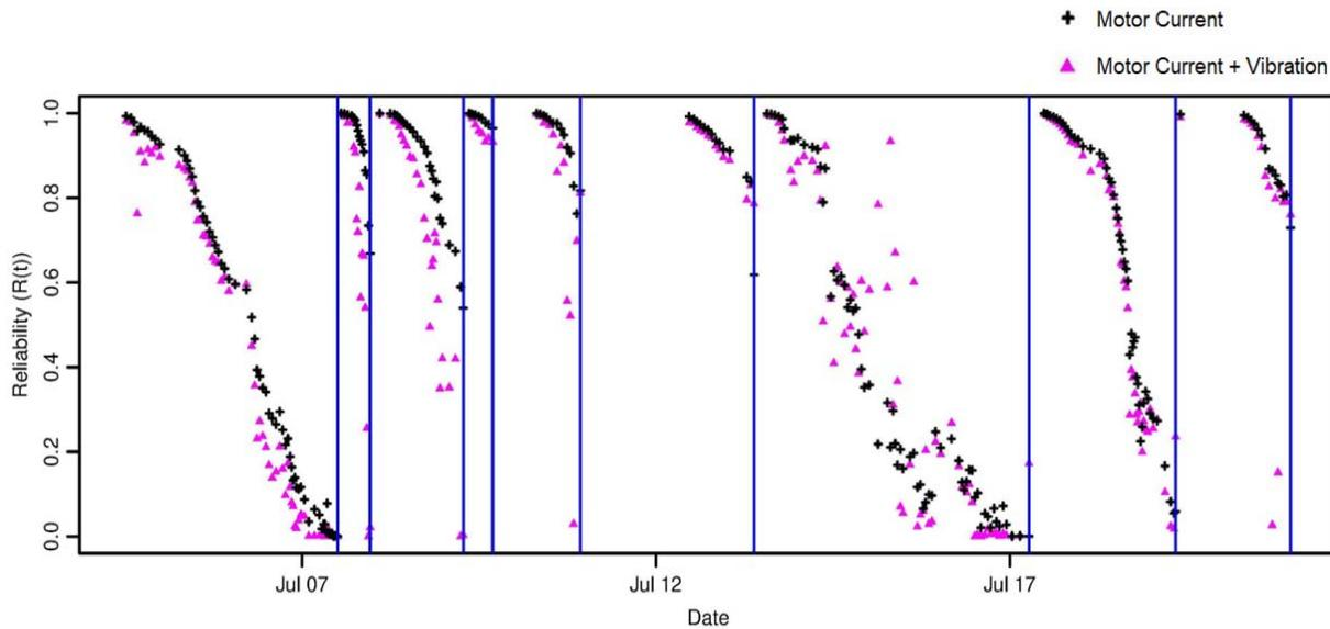
**Figure 6** Residual life of pump (9 ragging events) of station A. Black represents reliability of pump using motor current as a covariate and, magenta represents motor current and vibration parameters obtained from timewave data as covariates
