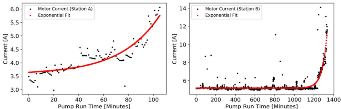
**Figure 3** Motor Current trend shown by black dot of station A (left) and station B (right). An exponential fit made to data is shown in red line.
