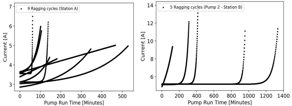
**Figure 4** Superimposed 9 ragging cycles from pump 1 station A shown in graph on the left, 5 ragging cycles from pump 2 station B shown on the right
