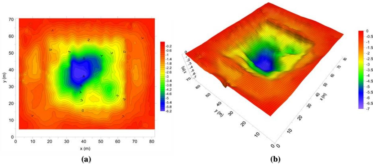
**Figure 3** (a) 2D and (b) 3D contour plots of water depth (depth from water surface till top of sludge) in the profiled Smart pond A. The colour scales indicate the water depth from the surface in metres.
