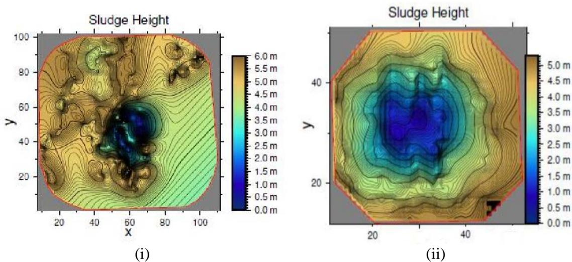
**Figure 4** Contour plots of Sludge distribution in Smart pond (i) pond B and (ii) pond C
