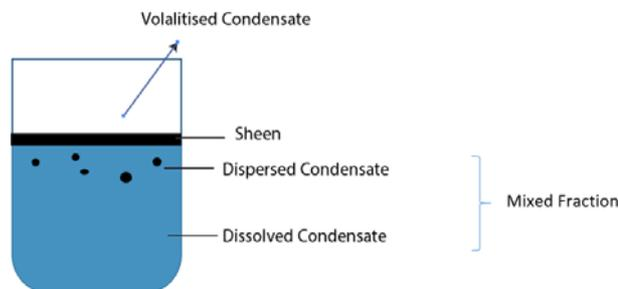
**Figure 1 Theorized oil components in water**
