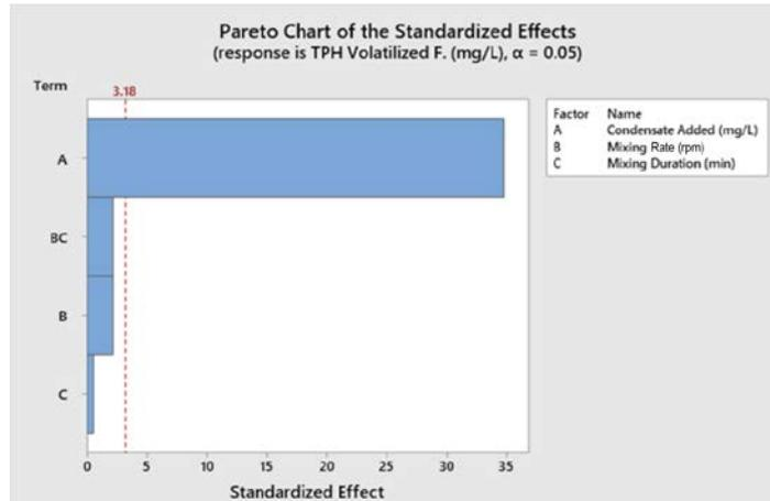
**Figure 4** Pareto Chart of Standardized effects for Condensate added (mg/L), Mixing Rate (rpm), Mixing Duration (min), for the TPH concentration in the Volatilized Fraction. Reference line for statistical significance ( $\alpha = 0.05$ ) is 3.18.
