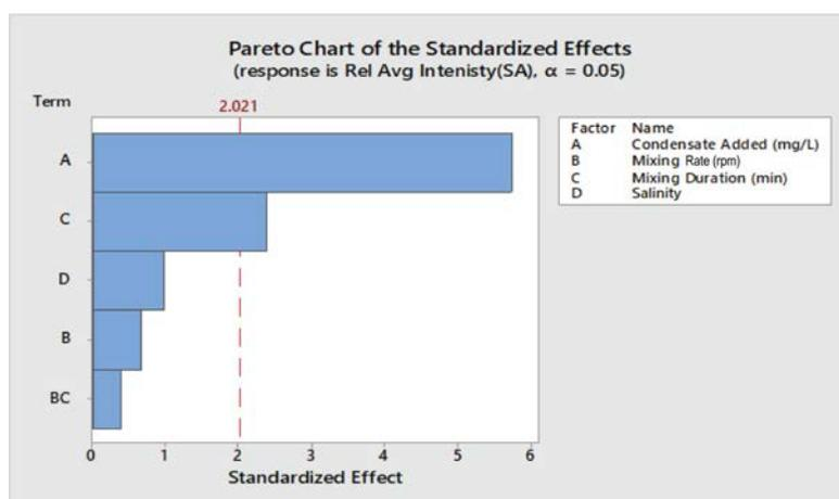
Figure 3 Pareto Chart of Standardized effects for Condensate added (mg/L), Mixing Rate (rpm), Mixing Duration (min) and Salinity. Reference line for statistical significance ( $\alpha = 0.05$ ) is 2.120.
