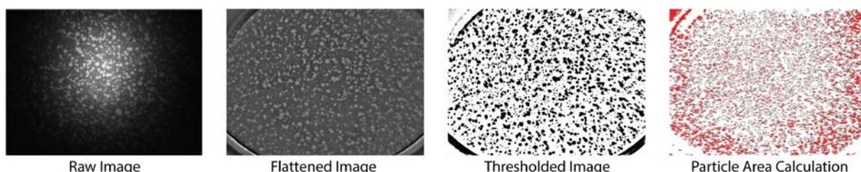
Figure 2 ImageJ processing of images to find sheen area of samples
