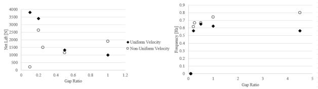
Figure 3 Vortex shedding frequency and lift force magnitude, for a uniform flow field (diamonds) and a non-uniform flow field (circles).
