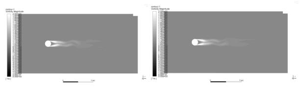
Figure 4 2 planes (with 4D separation) plotting vorticity contours, taken from a 3D model of a pipe far from the seabed, with a flow velocity of 2.5 m/s.
