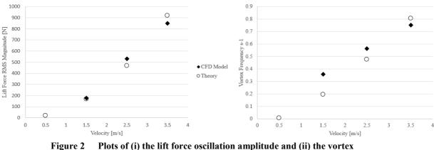
shedding frequency, for a 2D model with varying flow velocities.
