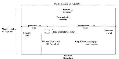
Figure 1 Model geometry and pipe positioning relative to the model extents.
