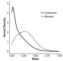
Figure 2 Observed probability density functions of ratio (*K*) for both blocked and unblocked pipes (2010-2016).
