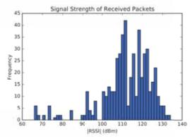
Figure 2 Received signal strength for the successfully transmitted particles for Bandwidth = 125 kHz and SF = 12
