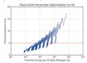
Figure 1Theoretical transmission distance and energy usages for all possible<br/>parameter combinations assuming a plane earth model with n=4<br/>and datasheet sensitivity. The optimum parameters for a desired<br/>distance of 5 km is the left most point on the horizontal line.
