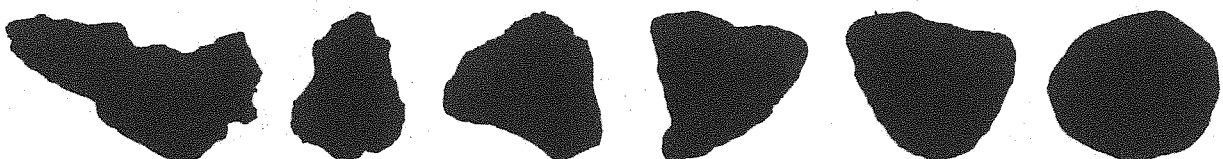
Figure 10: Typical Ore Shape at 2hr Time Intervals (0 - 10hrs)
