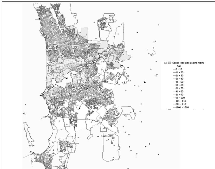
**Figure 2** GIS schematic showing the age of the piping networks within the Perth region.
