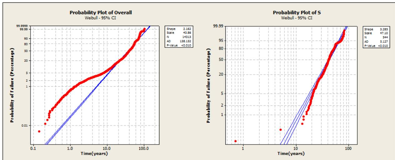
**Figure 2: A Weibull probability plot of all failures(left) and Steel(right) within the Perth Metropolitan Region**
