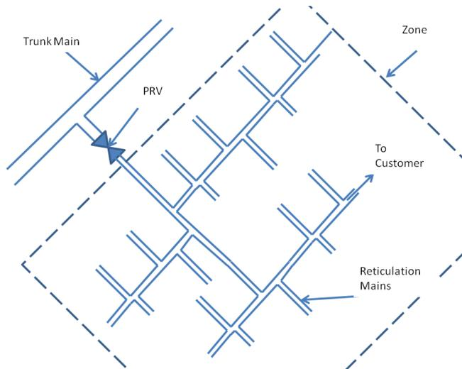
**Figure 1: Diagram of an idealised subsection of a water mains network.**
