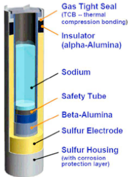
Figure 5: Diagram of the NaS battery (Wen, 2006)
