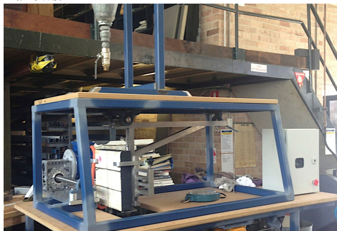
Figure 4 Newly Constructed DSRW Test Rig at UWA.
