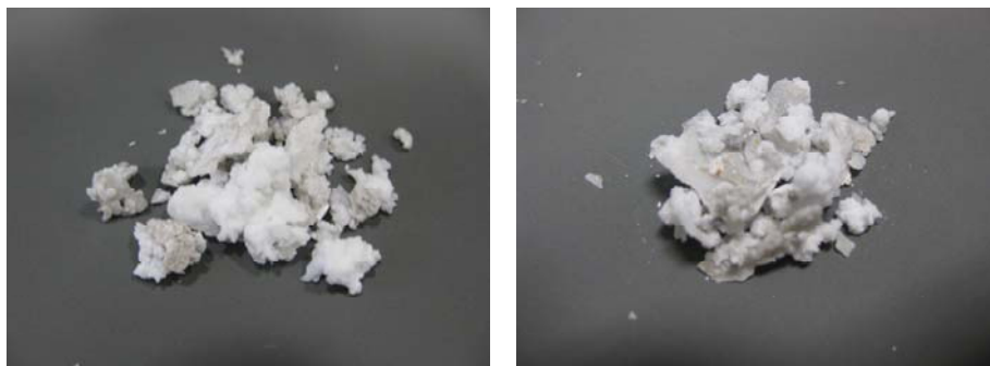
Figure 2: The collected precipitate from the surface of the mild steel plates in solution A (left) and solution B (right)
