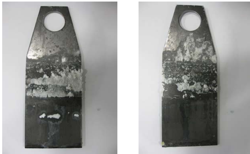
Figure 3: Precipitate formation on mild steel plates in solution A (left) and solution B (right)
