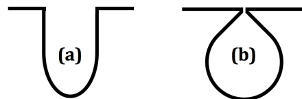
Figure 2 Different pit geometries. It is unknown if subsurface pits (type b) can be accurately measured.
